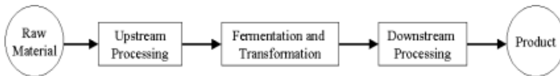
Figure 4. Notional Industrial Microbiological Process
